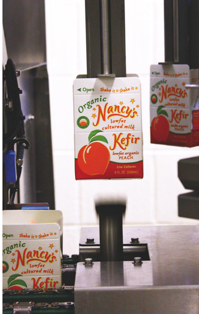
A vacuum arm (above) rises to meet a bottom-formed-and-sealed carton. The carton (below) is lowered to f/f/s machine's track.
